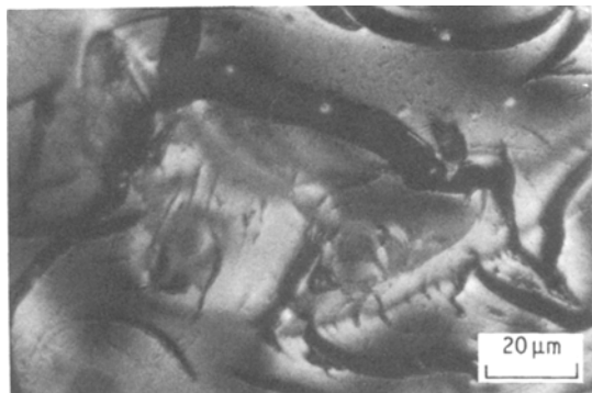
Figure 10 Optical micrograph of needle-coke HTT 1123 K. Note the fissure development in this domain.
